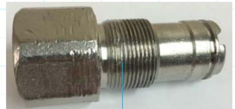
*Damage to threads on SDX III Nozzle*
